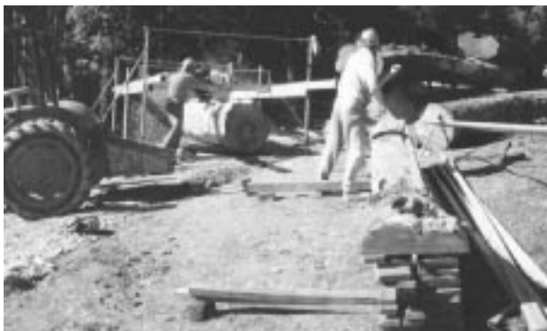
Frank Stries' modified Lucas saw, cutting a low grade eucalypt log for maximum recovery with high quality blackwood in the foreground.
